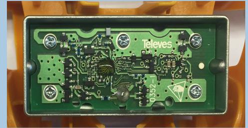
All Televés amplified antennas use the BOSS-TECH amplifier which actively monitors frequencies in the antenna range and applies auto gain control to allow maximum amplification across the entire frequency range. Less expensive, Chinese-made antenna amplifiers simply provide excess amplification which can actually make a signal less useful, while creating noise that can never be removed from the line.
