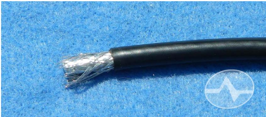
As gently as possible, fold the braid over to sit over the rubber sheath. It's perfectly normal to lose a few little wires during this process, but be as careful as possible. If you cut through the braid while cutting through the sheath, start over with a fresh cut.
