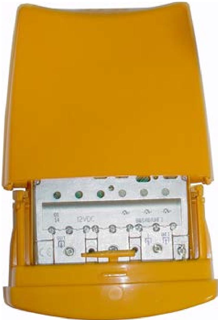
Televes' mast-mounted amplifiers are a little different from other amplifiers you'll find on the market. They're sort of a mix between preamplifier and distribution amplifier -- the power levels are extremely high, but then you have the ability to combine multiple signals and, at least according to the manufacturer, there's a higher noise figure than you normally find in a true preamp.
