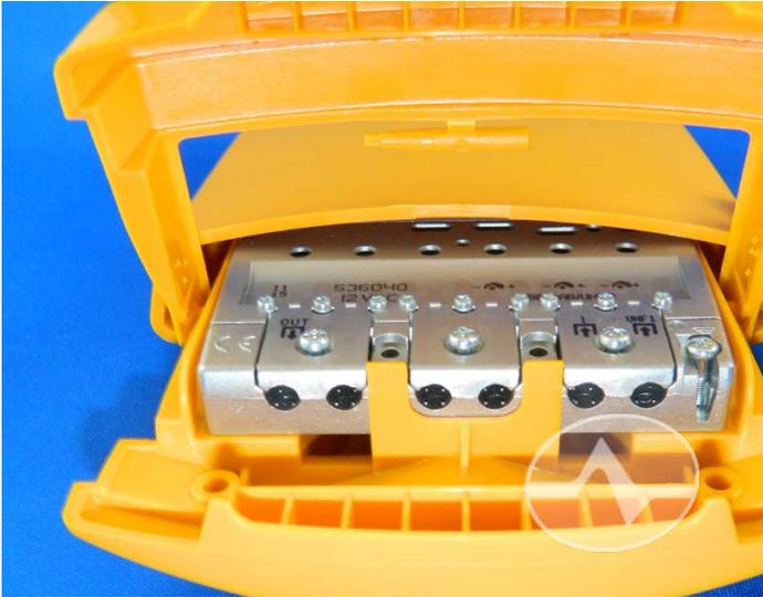
This is a view of the Televes 536040 Mast Amplifier. It's a general-purpose, 25dB amplifier that also combines two antenna feeds. Other mast-mounted amplifiers are very similar in the way they look.
