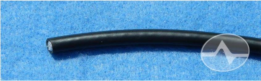
Start with a cleanly cut piece of cable. Pretty much any **cable cutter** will do here, but don't use needlenose pliers or "dykes" pliers if you can avoid it. A cable cutter with a curved blade will give a clean cut without pinching the cable down. That's less important with antenna cables than with satellite but it's still nice to start with a cleanly cut cable, as it makes everything easier.
