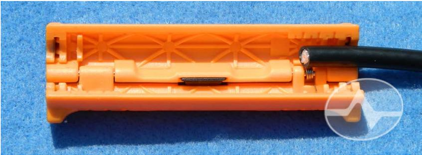
There are measurement notches in the tool. Lay the cable down so that no more than .75" of cable sits in the cutter past where the blades are. Close the cutter firmly and it should take no more than one full revolution with the cutter closed to cut the outer sheath.
