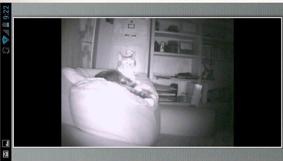
The PlugCAM has a ring of infrared LEDs enabling it to be used in full darkness. The image above was taken in a completely darkened room; the Android client is shown. A quick Google search seems to show that cats can't see infrared, so it's just a coincidence that the cat is looking at the camera.
