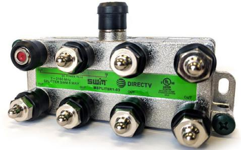
It is imperative that the proper splitters be used in order to accommodate the specific upstream and downstream frequency needs of SWM distribution. The [MSPLIT2](#), [MSPLIT4](#), and [MSPLIT8](#) splitters are designed for SWM distribution and are perfect for this use. Splitters may be cascaded if particular care is used to avoid excessive losses and keep the signal level higher than -55dBm at the receiver.
