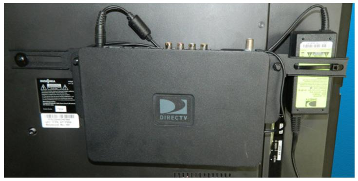
One of the easiest solutions to implement is to simply put a receiver behind every TV. This is usually the most cost-effective solution as it doesn't require special switching equipment. **DIRECTV H44 receivers** are small and light enough that they can stick to the back of a TV with industrial Velcro, or use one of Solid Signal's high-quality mounting solutions for a more professional installation.
