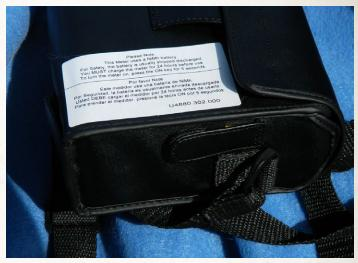
The underside of the meter shows the user-replaceable battery pack behind a plastic hatch. This battery is shipped installed in the meter and is similar to a cell phone battery where the batteries are shrinkwrapped together in plastic. These are NiMH batteries and so it's likely that over the course of several years their performance will degrade to the point where you will want to replace them.
