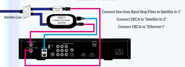
Use a green-label splitter and band stop filter as shown to connect the DECA to the HR20-100.
