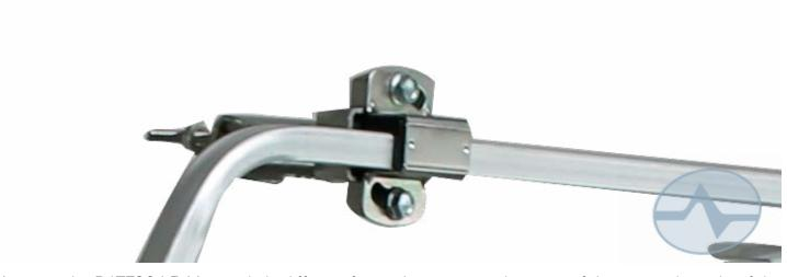
Mounting the DAT790 LR Mix is a little different from other antennas because of the size and weight of the thing. In other DAT790 antennas, the antenna mounts from a space behind the reflector. In this antenna, there are a pair of clamps that attach to the strengthening braces on the top and bottom. This allows the antenna to be mounted so it is balanced and this means it's likely to stay in place better for years to come.
