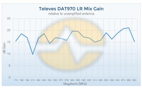
All tests were conducted at our laboratory approximately 55 miles from broadcast towers.
