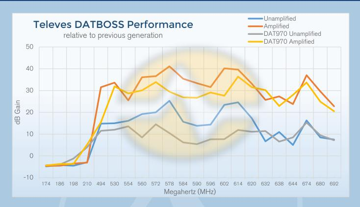
The DATBOSS shows superior rejection of VHF frequencies whether amplified or unamplified, just like last year's model. However, the new model shows significant improvements in both raw and amplified gain in the UHF range up to 620 MHz. This is the critical range since everything above that level will be used for LTE internet within two years.
