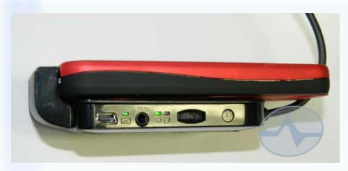
Probably the coolest accessory of all is the iOS adapter. It gives any 30-pin equipped iOS device the ability to connect to the Cinemizer. A Lightning version is coming soon.
