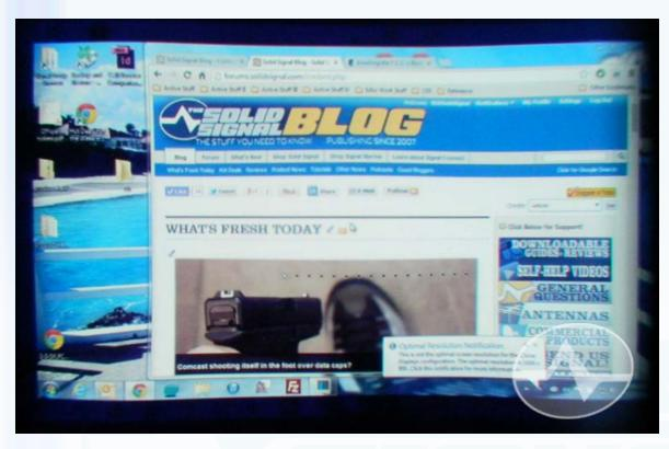
This is an actual shot of the view through the Cinemizer's optics. The native resolution of the two OLED panels inside the Cinemizer is 870x500. but it accepts inputs up to 1080p. The view was considerably sharper than
