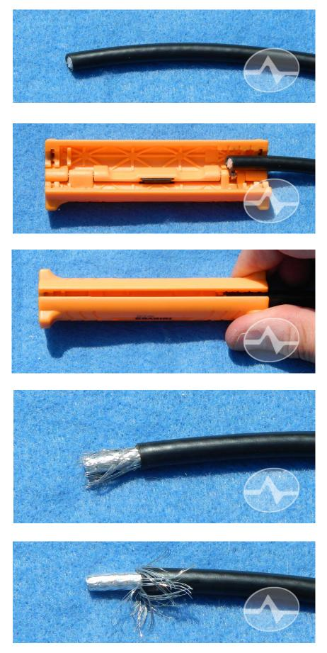
Start with a cleanly cut piece of cable. Pretty much any <u>cable</u> <u>cutter</u> will do here, but don't use needlenose pliers or "dykes" pliers if you can avoid it. A cable cutter with a curved blade will give a clean cut without pinching the cable down. That's less important with antenna cables than with satellite but it's still nice to start with a cleanly cut cable, as it makes everything easier.
