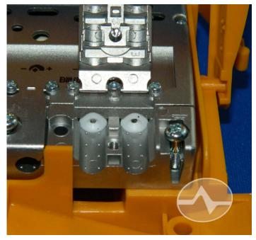
This is a view of the Televes 536040 Mast Amplifier. It's a general-purpose, 25dB amplifier that also combines two antenna feeds. Other mast-mounted amplifiers are very similar in the way they look.
