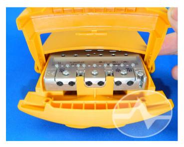
It's a good idea to get the amplifier wired and ready before zip tying it to the mast. To open the amp enclosure, firmly grasp it at its widest point and slide upwards. Even though the picture shows one hand (to make it easier for you to see what's going on) this is really a two-handed affair. If you grab the base with one hand, the top part will slide up easily with the other hand.
