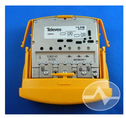
For those who want to use one or two antennas, the **<u>536040 Two-input amplifier</u>** is the best choice. Shown above, it lets you combine two antennas -- one UHF only and one UHF/VHF, and adjust the power level of the UHF/VHF antenna to help with any issues that can come with combining the two. For example, you could reduce the amplification of the UHF section of the UHF/VHF antenna and let the UHF-only antenna shine through.
