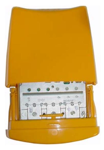
Televes' mast-mounted amplifiers are a little different from other amplifiers you'll find on the market. They're sort of a mix between preamplifier and distribution amplifier -- the power levels are extremely high, but then you have the ability to combine multiple signals and, at least according to the manufacturer, there's a higher noise figure than you normally find in a true preamp.
