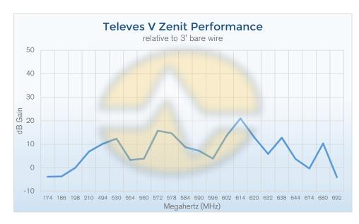
real-world testing, this typical for antenna was medium-rangeUHFantennas. VHF performance was poor but there did not seem to be active filtering of VHF signals. In a few frequency bands, performance actually surpassed any of the other mid-sized antennas but in other ranges it was adequate but not outstanting. For this test, a 3' length of bare wire was arranged in a dipole
