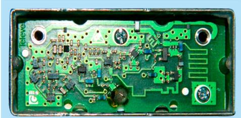
**Televes' BOSS amplifiers actively prevent control the amount of gain for every frequency.** This is a major upgrade in amplifier technology that only Televes has. Auto gain control allows every channel to be strongly amplified without worrying that other channels are going to be "overdriven" which would cause picture distortion or even damage to a TV tuner.
