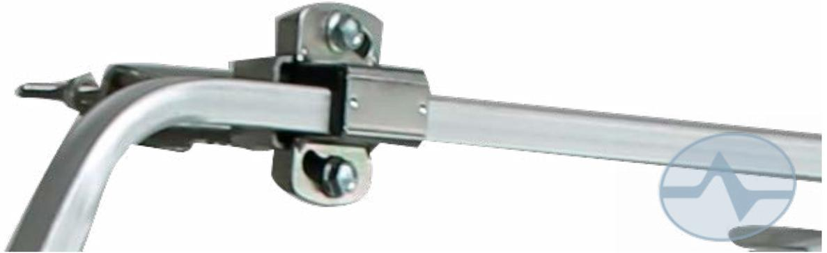
Mounting the DAT790 LR Mix is a little different from other antennas because of the size and weight of the thing. In other DAT790 antennas, the antenna mounts from a space behind the reflector. In this antenna, there are a pair of clamps that attach to the strengthening braces on the top and bottom. This allows the antenna to be mounted so it is balanced and this means it's likely to stay in place better for years to come.
