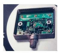
**amount of gain for every frequency.** This is a major upgrade in amplifier technology that only Televes has. Auto gain control allows every channel to be strongly amplified without worrying that other channels are going to be "overdriven" which would cause picture distortion or even damage to a TV tuner.
