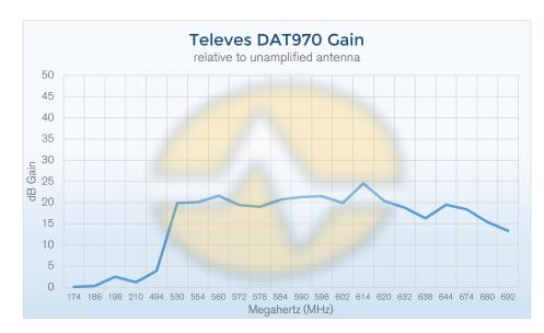
Performance on this antenna was more than satisfactory for an outdoor antenna and should be sufficient for most suburban installations. A truly long-range antenna would be better for much more distant stations. For this test, a 3' length of bare wire was arranged in a dipole shape and tested for reception. The DAT970s was placed in the same position and tested with amplification off and on. In both cases the power supply was in line, proving that the amplifier will perform with or without power.
