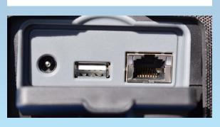
The AIM 2 gives you wired Ethernet instead of a largely symbolic USB type B port. The USB port can still be used for firmware updates but the USB type B connector is now gone. Once upon a time there was hope that the type B connector would be used to enable direct upload and download from the meter, but the proper procedure has always been to use the included flash drive. That procedure has seemed a little archaic in recent years.
