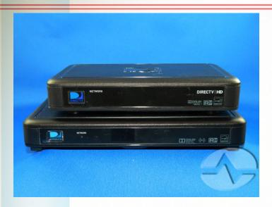
At first glance, the C41W (bottom) looks just like a C31 (top) until you realize it doesn't have a coax input. It is wider and not as tall. The power button design is different, with a bit of thick clear plastic between your finger and the logo. From the top it's very obvious that the C41W is larger than the C31, but not by much.
