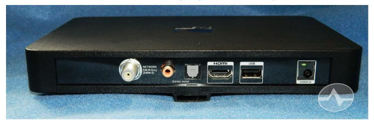
The good news is that the C61K has a full complement of outputs. The HDMI output is fully HDMI 2.0/HDCP 2.2-compliant, and there are both optical and coaxial digital outputs. DIRECTV puts a USB port on everything, and in this case it won't do much for the software. It's a convenient place to plug in the power from a streaming stick, and that's about it.
