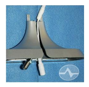
Personally, I recommend using this booster on its supplied stand. I'm not a big fan of sticking things to the window. But that's completely your call. If you want to use the supplied stand, start by feeding the cable ends from the booster through the top. Don't try to push them through the slot, they are too thick. Instead, thread them through the top and slide them all the way to the bottom.
