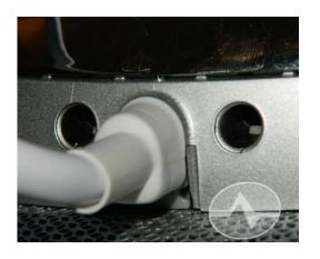
The cord will pass through the widened area at the bottom of the stand. If you want to, use an adhesive strip at the bottom of the base to keep the amplifier attached to the window sill (see the next page.)
