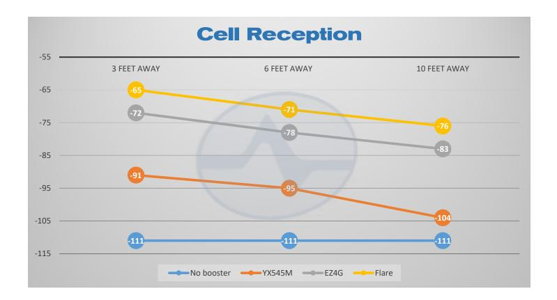
The test regimen was simple. I tested voice performance with no booster, with an ancient zBoost YX545M (which was one of the most powerful budget boosters at the time), and against the **SureCall EZ4G**. Test data for a booster-free environment and for the YX545M were consistent with prior data, so I used prior measurements for EZ4G.
