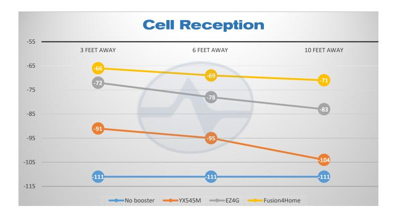
I tested the Fusion4Home against the SureCall EZ4G and the YX545M that is usually in place in our lab. The results were phenomenal. What you need to know here is that I actually had to do the test multiple times because the Fusion4Home had so much power that it was automatically cutting itself back.
