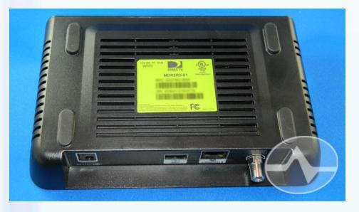
Not a whole lot to see on the underside, except a label calling this an MDR2 (The original was an MDR1) The original GenieGO has keyhole slots on the back so you can mount it on a wall, but this one doesn't.
