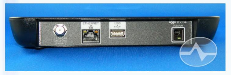
Here's the big difference: GenieGO 2 has a coaxial connector. That's right, it can be connected by **coax OR Ethernet**, whichever works best for you. This means it doesn't need to be in the same room as your router or switch. You can connect it inline with any DVR or receiver. Also, there is the customary USB port for you to add a flash drive for almost unlimited storage.
