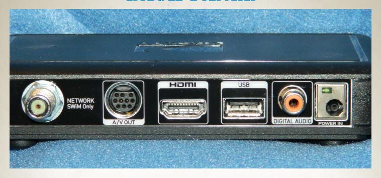
Even though this receiver is tiny, there's a lot going on behind it. Of course, there's a coax input. Because the HR34 is SWM-only, and because you need an HR34, this box is SWM-only too. The next connector is for a component or composite connection. Our <a href="https://example.com/H2510PIN"><u>H2510PIN</u></a> dongle for H25s works fine, and there will be one for composite as well.
