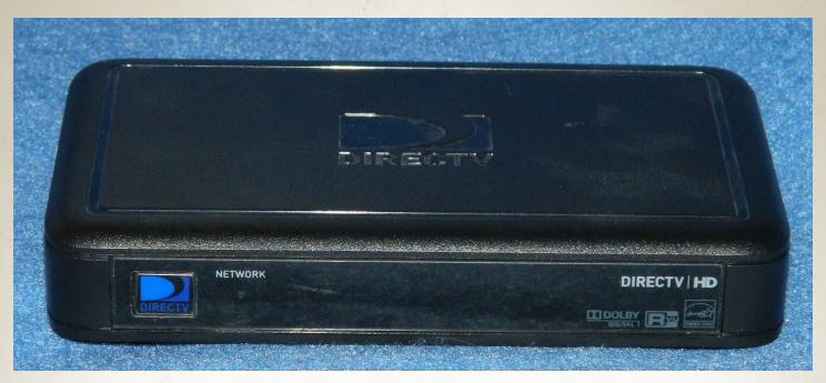
There's not a lot to look at with this little box. The front panel has one button on it. Quite a change from the old days when there were 15 or more buttons on the front. It will work with an RF or IR remote, but you do have to use a remote. The power button lights up when the C31 is in use. To the right of it is a network light that glows green when the C31 is connected to an HR34.
