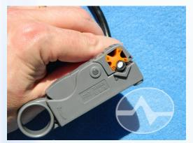
If it's not a 6, gently push the orange plastic block out of the tool and rotate it, then put it back so it looks like the picture.
