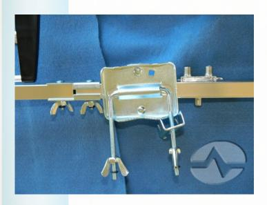
The arm with the combiner goes at the bottom of the antenna, and the combiner goes on the underside (so that when everything is assembled, it will be at the front.) Also, the wingnuts at the edges should point toward the bottom.
