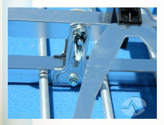
Tighten the wingnuts to keep the antenna separated from the reflector.
