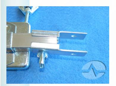
First remove one of the two wingnuts in the hinge. The hinge is the part closest to the center. In the photo at the top, it is on the right.
