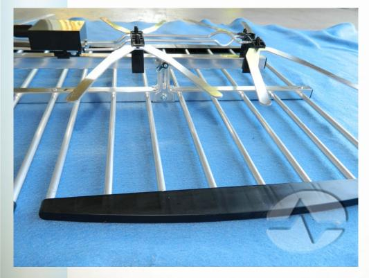
Both should arms attach to the antenna assembly as shown below. Once you have one side done, start on the other side. It may be helpful at this point to loose the hinges so that one assembly sits on a flat surface while you attach the arms to the other assembly. If you do that, tighten the hinges back up so that it's easy to lift the antenna when you are done.
