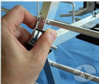
The back end of the antenna (where the elements are most tightly spaced) has a wingnut and bolt. Remove these two items and set them aside.
