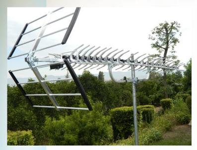
Mount the antenna on a mast by sliding the mast mount over the mast and tightening the clamps onto the mast. Attach your antenna cable to the bottom of the antenna, using the supplied weatherproof boot to shield the connection. The cable can run through the plastic cable clamp on the mount.
