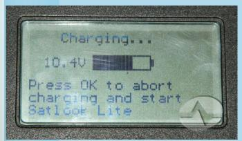
Before you even start to align the dish, the first thing you'll want to do is charge the meter. The first time you get it, it will take up to 12 hours for a full charge. When you plug the meter in, you should see this display (shown at left.) indicating that the meter is charging. If you don't see this display, or if the meter boots up by itself, that could be an indication that the battery got loose in
