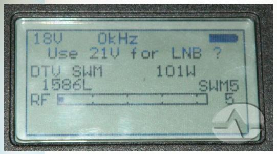
Turn on the meter by pressing and holding the OK button. After it initializes, it will go straight to the Satellite Search screen. If you have already used the meter, it will go back to the last satellite you were
