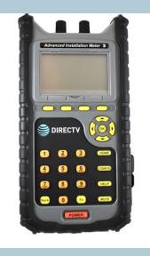
A good satellite meter is critical to any successful installation, and a professional should never depend on the signal meters built in to a DIRECTV receiver. Inexpensive signal finders do not work with SWM distribution, so it's best to get the meter you'll need.
