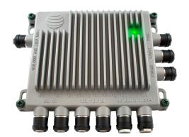
The SWM-30, also known as the DSWM30, is the current generation DIRECTV multiswitch. In most installations, it will support two banks of 13 tuners each, 26 tuners in total.
