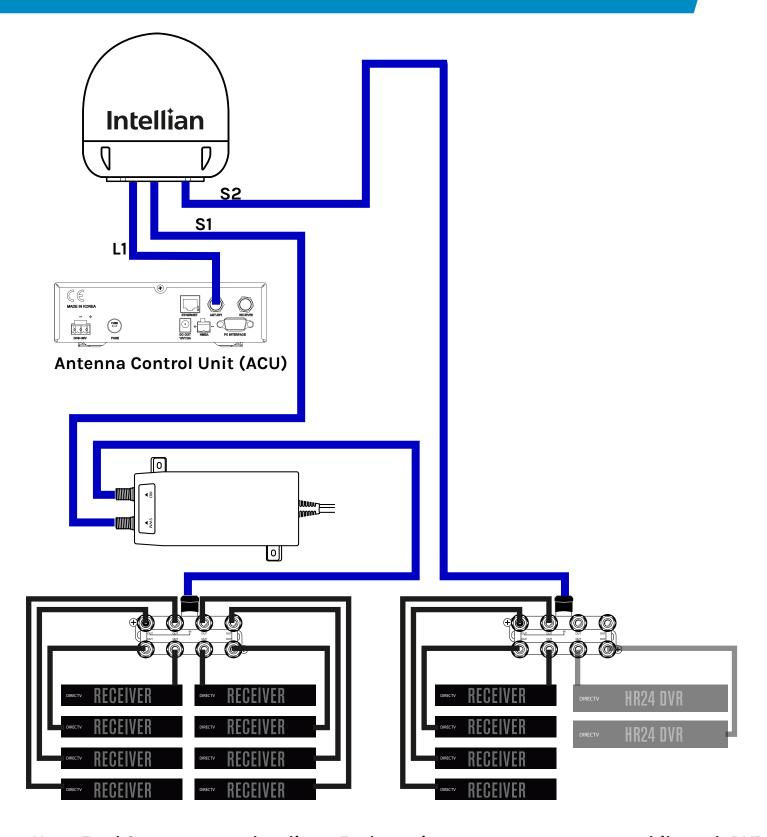
Note: Feed 8 tuners to each splitter. Each receiver counts as one tuner, while each DVR counts as two tuners. A total of 16 tuners are supported in the basic configuration.
