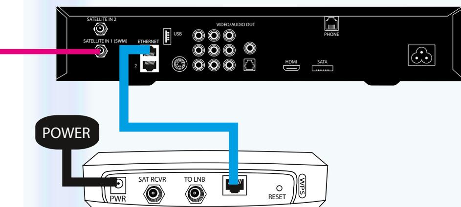
With your receiver powered up and connected, connect the CCK to "Ethernet 1" and use:
